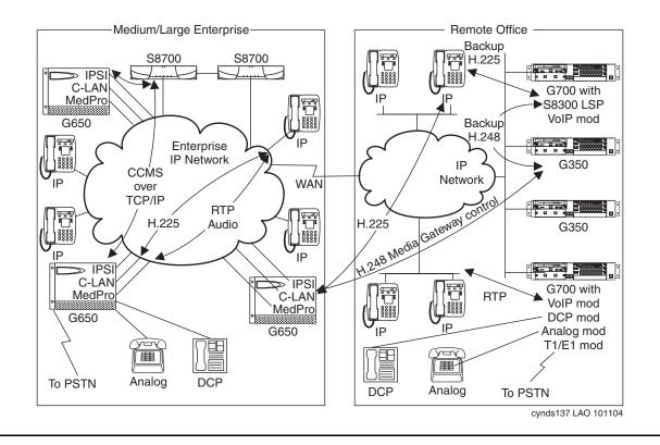
Figure 37: S8700-series IP-PNC with remote G700 or G350s
